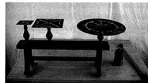
Fig. 5: Chladni figures, experimental setup, method published by Ernst F. F. Chladni 1787.
