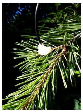
Figure 3. Self-built piezo needle sensor.
