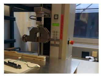
**Figure 5**. Finger pressing force sensor evaluation with the compression test machine. The steel peg has a diameter of 10 mm and a spherical tip. In this picture, the tip applies a controlled force to position P2 of the key.
