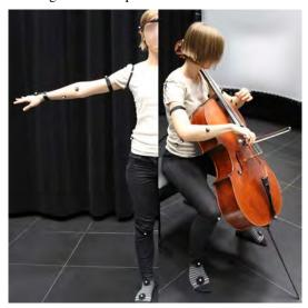
**Figure 2**: The Musician wearing passive reflective markers used for kinematic motion capture. Note the markers on the back of the hands (RFIN/LFIN), the tip of the bow (CLTP), the elbows (RELB/LELB), and the forehead (HDFR)
