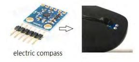
Figure 7. GY-273 electric compass on a cap.
