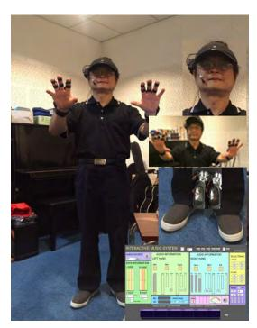
Figure 1. Musfit, a prototyped wireless integrated wearable interactive music system
