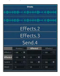
**Figure 3**. An example of a TC loaded with audio processes in I-SCORE. Selecting a particular process shows a complete widget for editing the relevant parameters. On a single TC, there can be only a single Mixing process (the table at the bottom), but there is no limit to the amount of other processes i.e there can be multiple sound files, etc.
